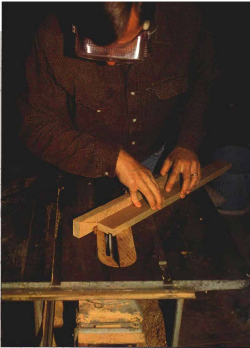
The trick to properly spaced slots is an indexing stick. The author attached the indexing stick to the miter fence on his table saw and set the small index pin, which is visible at the left of the stick, into the last slot cut, thereby perfectly aligning the piece for the next dado cut.
